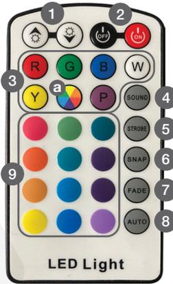
1.  $\uparrow/\downarrow$  (+/-): Adjust speed, brightness, or sensitivity depending on the function the unit is set to.
